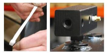
134. Fit a ¼ BSP blanking plug to the hole at the front of the fountain using PTFE tape, tighten.
