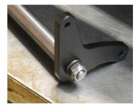
Insert the weighshaft through the bushes in the motion brackets - reach rod lift arm goes on the right hand side of the chassis.
