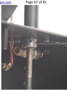
158. Apply a liberal smear of grease to the brake screw as shown and thread into the brake nut far enough so that an M10 nyloc nut can be fitted on the end to stop the brake being unscrewed off its nut in use. Grease the rear face of the brake nut and one face of its thick washer and assemble with an M6 x 12mm bolt. Check that the brake nut can slide in its slot when the retaining bolt is fully tightened.
