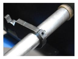
23. Attach the brake pull bar to the brake link centre via its elongated slot and the clasp at the top of the brake link centre. Rotate the brake cross bar so that the two components are linked together. The shaft of the brake pull bar should be left pointing towards the front of the chassis.
