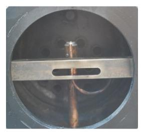
121. Push the smokebox dart through the door as shown, slide an inner handle over the square shaft and screw on the outer handle - don't tighten it up at this stage.
