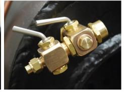
Adjust until both fittings are exactly in line with each other, ensure that both are positioned the same distance from the backhead.
