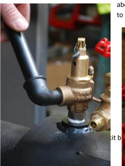
above, the exhaust vent should point to 10 o'clock as shown. Once correctly
