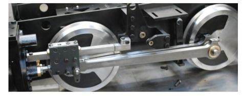
64. Check that the piston is 6.5mm from the end face of the cylinder – a vernier caliper or steel rule can be used. To adjust, loosen off the piston rod locknut at the crosshead and turn the piston rod – it has machined flats for a 9mm spanner. When the piston is in the correct position, tighten the locknut.
