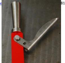
Attach the reversing lever trigger link using an M4 x
