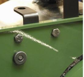
170. The important thing to remember when fitting the saddle tank it to get it the right way around! You can't go wrong, the mounting bushes at each end are at different spacings - find the end that matches the pair of angle brackets already fitted and you've got it.
