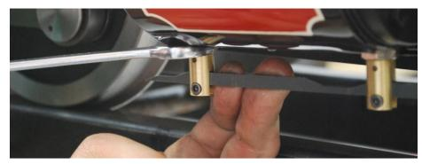
operate freely, they should require next to no force to pull the handle at the footplate end.
