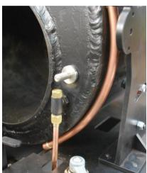
147. Fit 10mm unions to each valve chest using PTFE as shown. Fit the left hand steam pipe (longer one) into its union in the left hand valve chest, right hand (shorter one) to the right hand steam chest.
