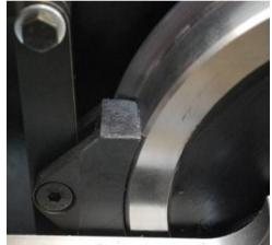
27. Attach the rear brake lever to the allocated slot on the side of the brake rod in the alignment that means it does not rotate in parallel with the brake link centre. If fitting is tight use an M8 bolt and several washers, gradually tighten to draw into place then remove and fix with an M8 x 20 bolt and washer.
