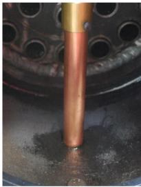
119. Fit the smokebox blower fitting (5/16 x 32 thread) to the left hand side of the smokebox - fitting on the outside with pipe connection facing rearwards, nut on the inside. Connect the blower pipe as shown, with its end alongside the blast pipe, facing up the chimney.
