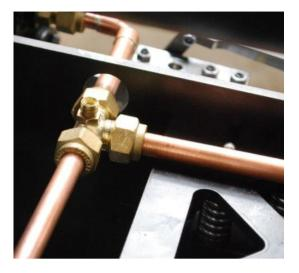
149. Attach an 8mm compression union to each steam valve with PTFE tape.
