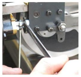
66. Remove the valve chest and cover. Coat the valve face with cylinder oil. Apply a valve chest gasket (green side up) to the valve Face, ensuring all holes line up. Apply more cylinder oil to the top of the gasket and replace valve chest – circular steam pipe boss goes towards the centre.
