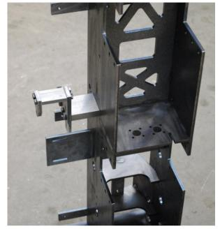
the buffer beam fits either way round so you can spray either side black and call it the back. The drag beam has an 11.8mm hole for a vacuum brake connector if fitted - this hole goes on the right hand side which determines which side of the drag beam is the back.
