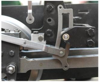
84. Attach the front end of the radius rod to the combination lever using an M4 x 20 motion pin as shown.
