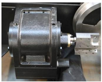
32. Fasten the complete cylinder assembly to the chassis using ten M6 x 16mm hex head bolts (13Nm). Valve chests face downwards at this stage, remember the cylinders are handed, the pistons rods face towards the back of the engine.
