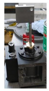
Run an M8 half nut down the piston rod, then fit the right hand crosshead - don't tighten the nut at this stage.
