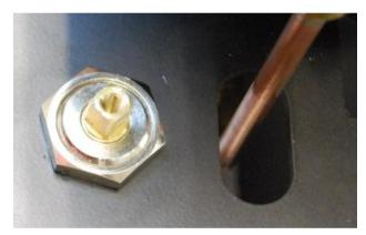
145. Fit the water valve to injector pipe as shown to each water valve.
