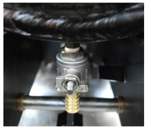
153. Screw the upper water gauge fitting into the backhead as shown using PTFE tape. Repeat for the bottom fitting.
