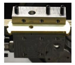
51. Crosshead cover plates are handed - select the left hand one, shown below, and put the gudgeon pin through its hole in the bottom corner. Place a drop link spacer and drop link over the gudgeon pin, and temporarily put an M5 bolt in the centre hole as shown to align the parts as shown.
