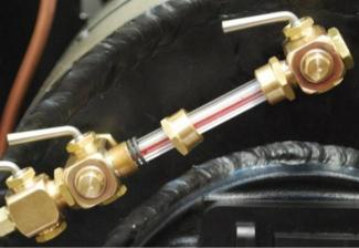
155. Fit the water gauge blow down pipe as shown - bottom end goes through a small hole in the left hand footplate, next to the injector water valve.
