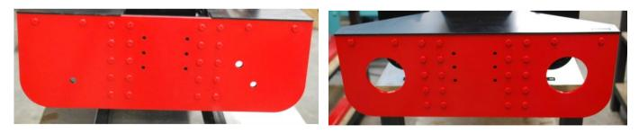
110. If not previously assembled, attach drag beam and buffer beam to the chassis. The buffer beam has two large holes in it to allow removal of the pistons for maintenance. Attach using 24 off M6 x 16mm hex head bolts, fit to all the holes except the six coupling mounting holes shown in the middle of the Beam. Attach the drag beam in the same way using 24 off M6 x 16mm hex heads to the twenty four holes except from the six inner holes.
