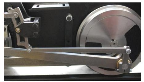
tighten both then back off half a turn to provide running clearance.
