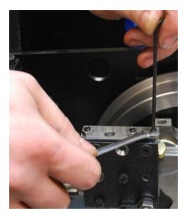
55. Slide the crosshead up to the cylinder rear cover and lightly nip up the M5 hex head bolt attaching the guide bar to the cover. Slide the crosshead to the opposite end of its stroke and repeat for the mounting bolt at that end as shown. Slide back and forth to make sure the crosshead slides freely on the guide bar, then fully tighten the fixings.
