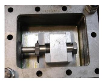
99. Roll the engine forwards to front dead centre and check that the front edge of the slide valve is just opening the front port.
