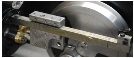
mounting block with two M5 x 20 hex head bolts - don't tighten at this stage.
