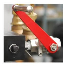
143. Fit the safety valve to the bush at the front of the firebox on top of the boiler. Use a steel adaptor ferrule with PTFE tape - tighten into the boiler with a 22mm spanner, then screw the valve itself onto the ferrule, tighening with a spanner. When viewed from
