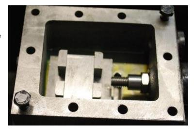
71. Push the valve rod, through the drive block and lightly clamp in place with the other lock nut.
