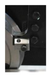
49. Grease all faces of the guide bar and place in the crosshead slot.
