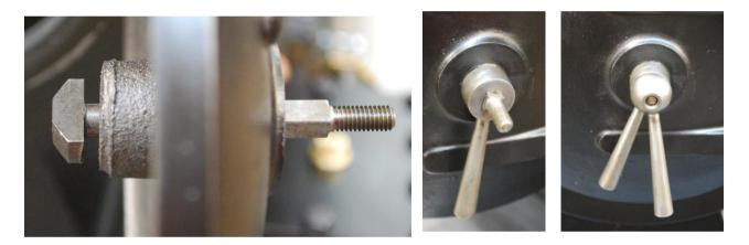
122. If fitting vacuum brakes, put the ejector exhaust fitting into the hole in the right hand side of the smokebox, pipe fitting facing rearwards and secure with an M8 nut on the inside. If not, then blank off the hole with an M8 x 20mm hex head bolt.
