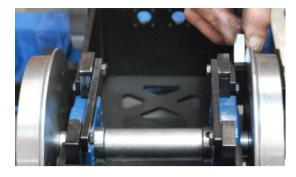
15. Grease all four crankpins. Turn the wheels so that the crankpins all face to the rear as shown, then fit the left hand coupling rod - flange of its bush faces the wheel, oil wells face downwards.
