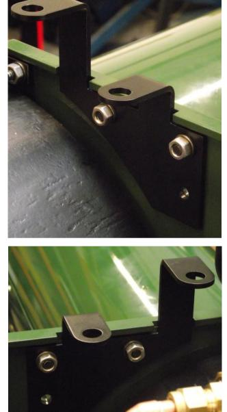
168. Fit two saddle tank brackets to the smokebox with M6 a 16 bolts and nuts - don't tighten at this stage.
