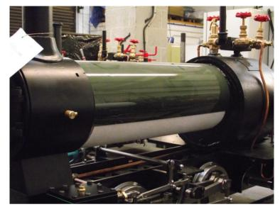
161. Temporarily hold the two sheets tightly together, ensuring that the ends of square to the smokebox and tubeplate - you can use ratchet straps to do this, or a helper can hold top and bottom. Drill through the fastening holes in the bottom sheet straight through the top sheet with a 3.2mm drill - **don't drill into the boiler, if in doubt, fix a stop collar on the drill so that it can only penetrate a short distance**. Fix the two cladding sheets together with 4mm self-tapping screws.
