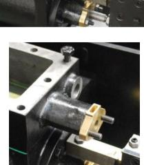
69. Fit the valve rod, complete with clevis, passing the threaded end through the gland and into the valve chest. Run a slide valve locknut onto the end, hexagonal head nearest the boss as shown.
