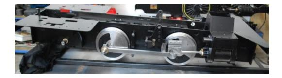
44. The rear end of the drain cock operating rod is fastened to the right hand frame with an M6 x
