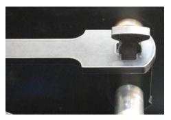
24. Place the brake cross bar under the brake pull bar with holes lining up. grease the brake barrel pivot and insert from underneath - secure with an M8 x 25mm hex head bolt fitted from underside.
