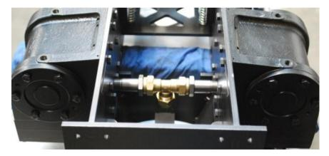
positioned, tighten both nuts up fully which will crush the olives onto the exhaust stubs, making a steam-tight connection.
