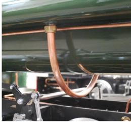
175. Fit the pressure gauge to its bracket and connect to the fountain as shown.
