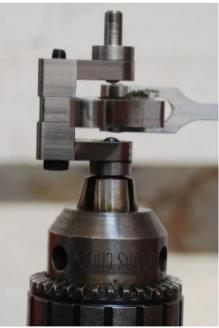
81. Fix the expansion link trunnion pins as shown using Loctite243 - hold in a drill or lathe chuck to tighten.
