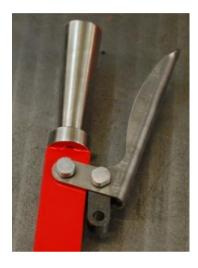
90. Attach the reverser latch lifting links to either side of the reverser lever latch using M4 x 20 motion pins as shown, ensure that the holes used in the reverser latch lifting links are the ones at the end of the shorter shafts so that the remainder of the part can situated so that it is parallel with the Reversing lever, attach via a M4 x 20mm motion pin, from the front and nyloc nut.
