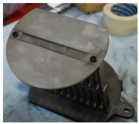
132. Fit the back head, grate and baffle combination into the fire box in the rear of the boiler and secure with the pair of stainless steel backhead knobs as shown.
