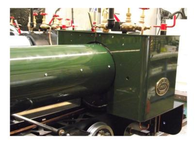
165. Join the two cab sheets with brace piece in front of the safety valve, fix with M6 x 16mm bolts with a washer and nut inside the cab. Tighten nuts and all footplate bolts.
