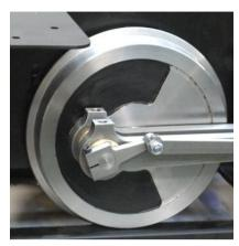
98. Set the slide valve using the adjuster nuts so that its back edge is just opening the rear port - there should be a tiny crack of a black line showing as the valve uncovers the port with the wheels set at back centre.
