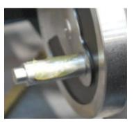
16. Turn the wheels so that the crankpins are at the front dead centre position as shown. Using a square, set the front axle's front hornblock square with the bottom edge of the frames and tighten its three securing bolts with the hornblock lightly pushed up against the axlebox. Turn the wheels to back dead centre, push the rear hornblock up against the axlebox and tighten its fixing bolts.
